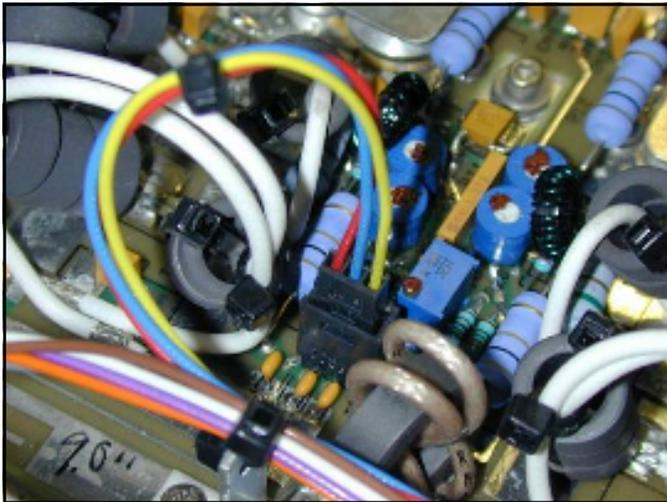
Gate bias/alarm connector & over temp
